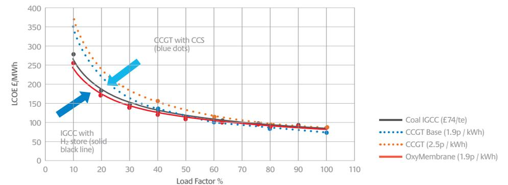
CCGT with CCS is compared to an IGCC with a H<sub>2</sub> store. ‘Oxymembrane’ means H<sub>2</sub> from methane by precombustion, with separation assisted by membrane (Cachet as noted above).
