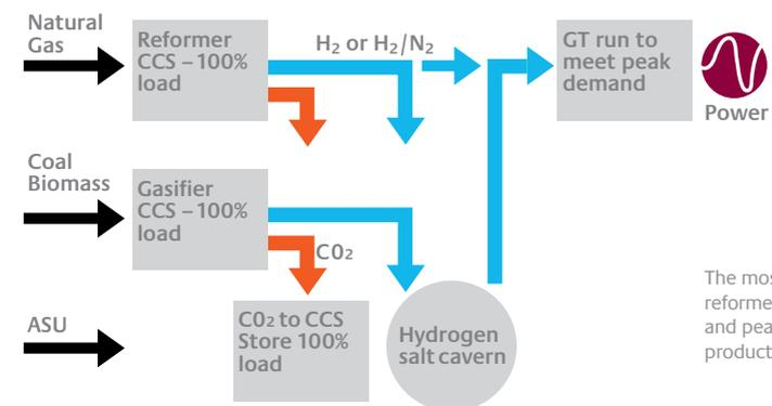
The most expensive assets (gasifier, reformer, CCS) all 'sweat' at 100% load and peak efficiency, even though power production varies.
