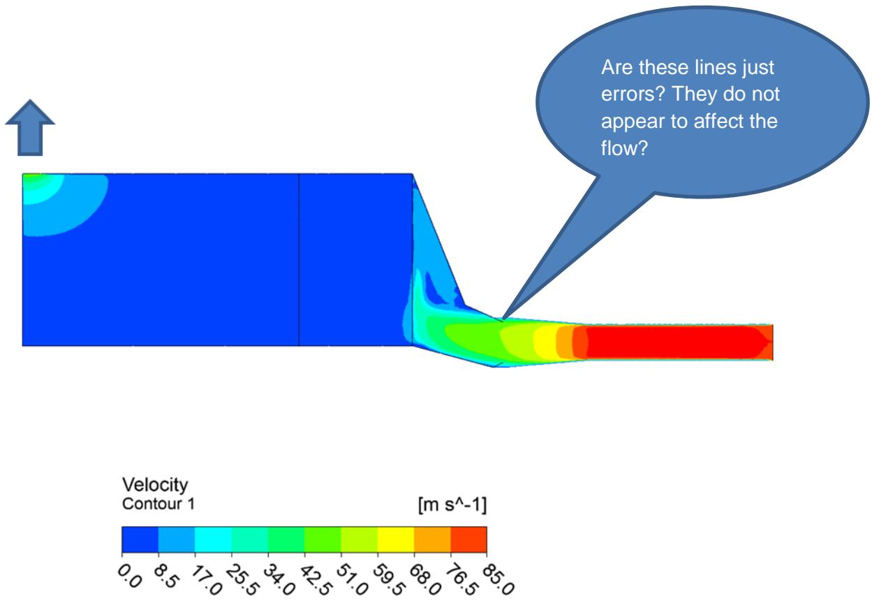
**Figure 3:- CFD simulation showing predicted velocity contours along the central plane of the HRSG (Open topped).**
