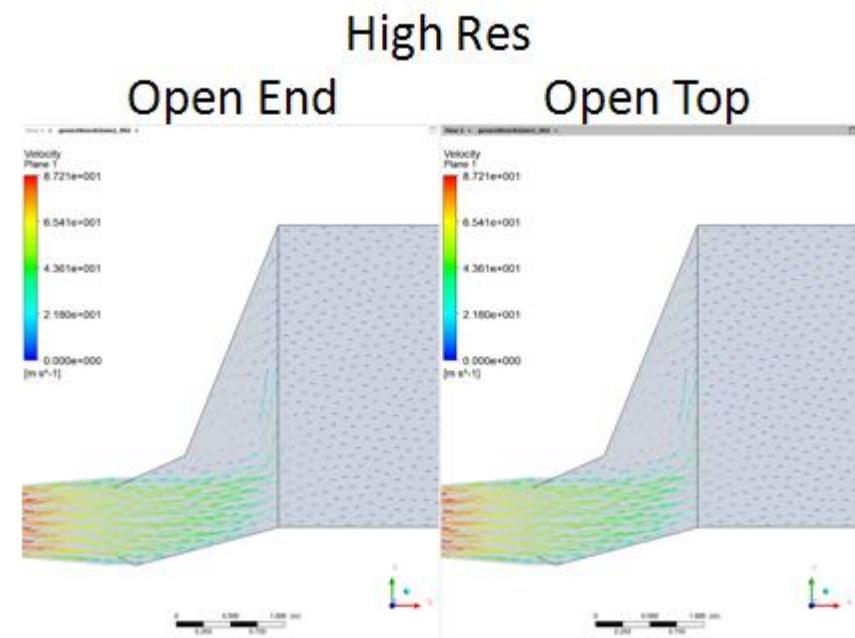
**Figure A6c:- Side on view showing velocity vectors along the central plane for both the open end and open topped cases.**
