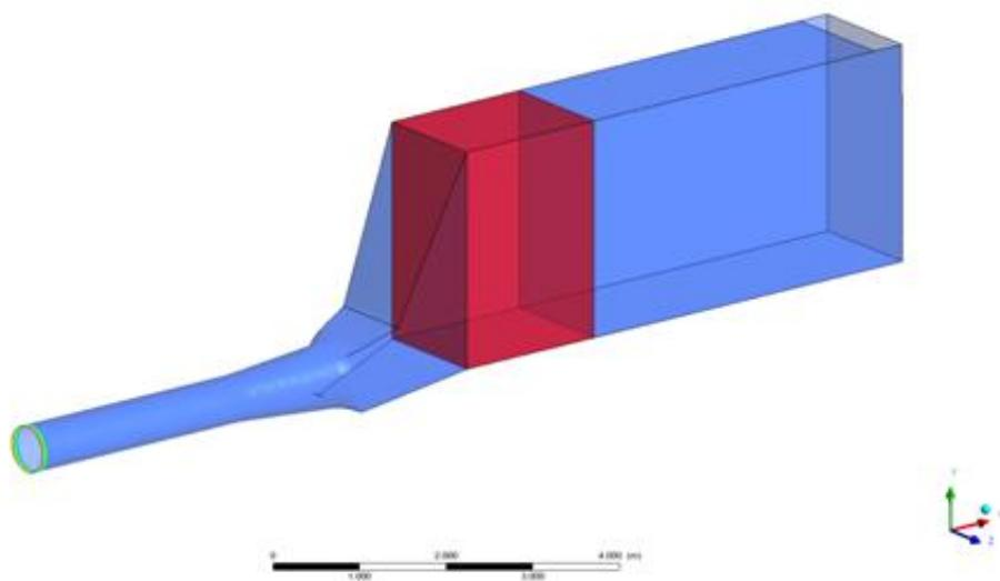
**Figure A2:- Geometrical representation of the scaled HRSG, taken from the design drawing Figure 4 of the BoD.**
