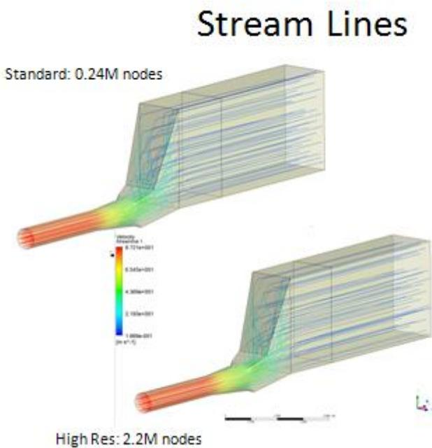
**Figure A5:- Streamlines illustrating the flow pattern through the HRSG (Open ended).**
