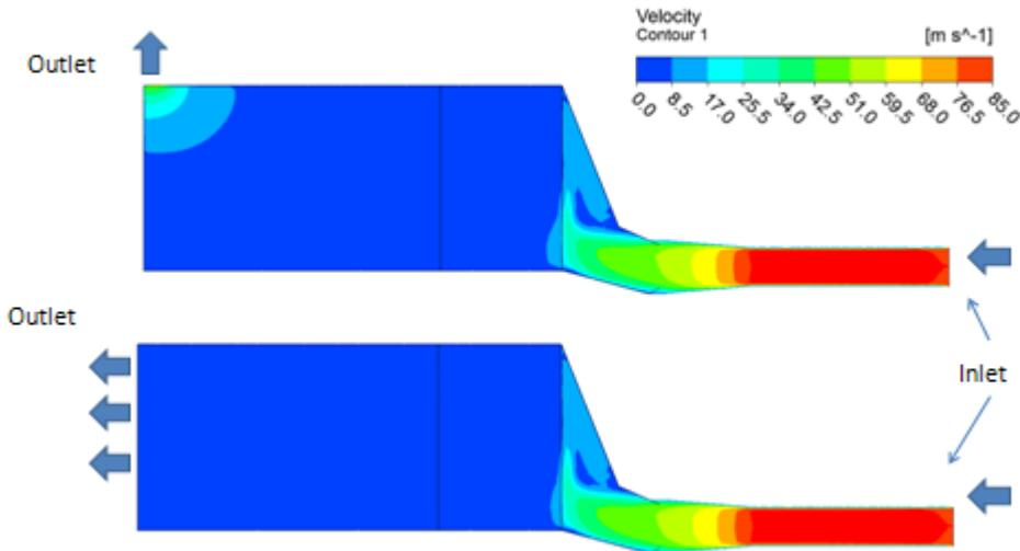
Conclusion: configuration of outlet has little effect on flow upstream of heat exchanger
