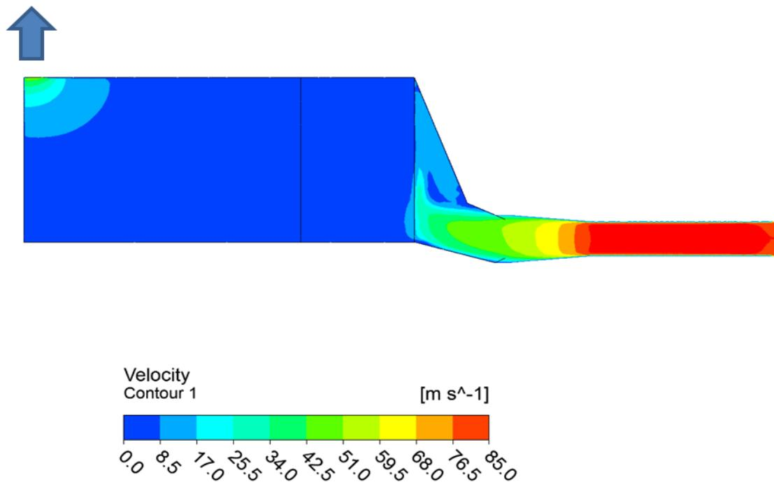
**Figure A6d:- Side on view showing velocity contours along the central plane for the open topped case.**
