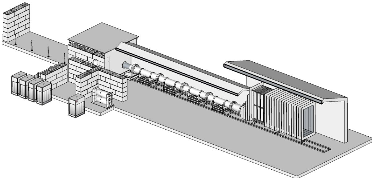
**Figure 10:- Physical layout of the ETI rig with HRSG extension**
