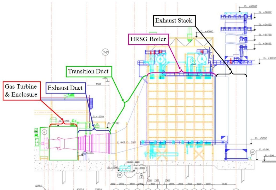
**Figure 1:- GE 350 MW CCGT.**
