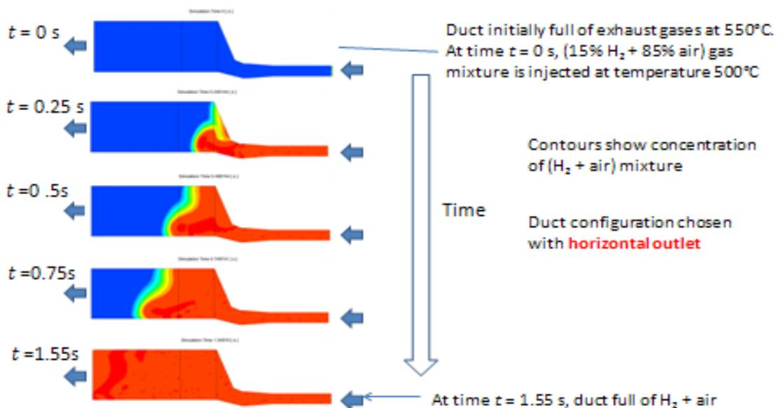
Figure A9b:- Time varying gas concentrations for the open ended case.
