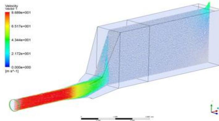
**Figure A6a:- Velocity contours through the HRSG with the end sealed and an open top (central plane).**
