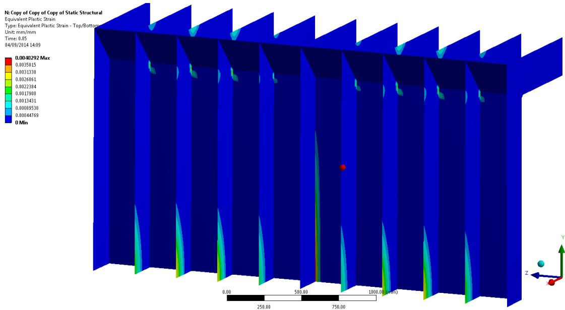
**Figure 7:- HRSG Strains for a static load of 8.5 barg.**
