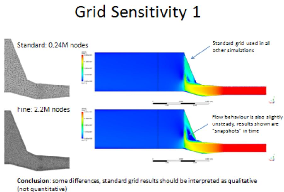
**Figure A4a:- Grid sensitivity results (Velocity contours open ended).**
