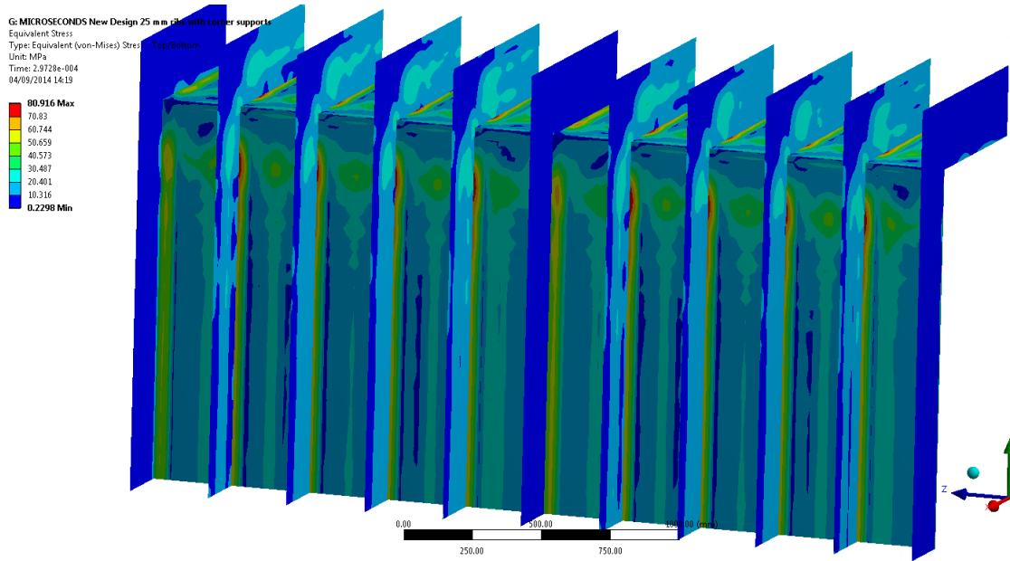
**Figure 9:- HRSG stress analysis (Von Mises Criteria) for a dynamic load of 104 barg.**
