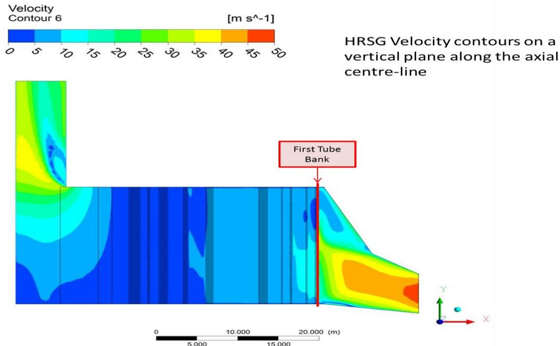
**Figure 2:- Velocity distribution through typical heat exchanger [Courtesy of D. Abbott].**
