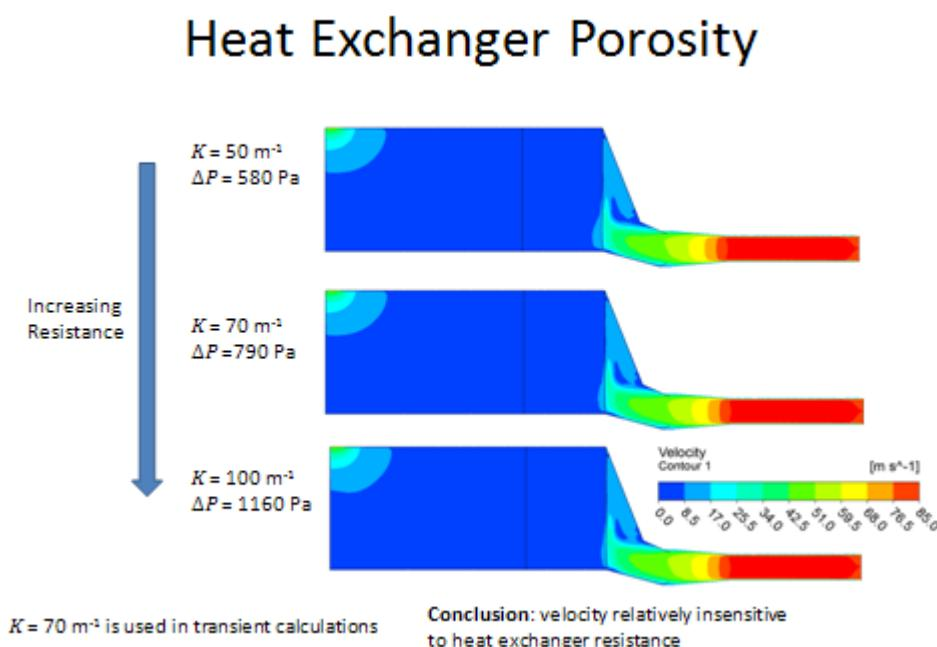
Figure A7:- Influence of assumed heat exchanger porosity (Pressure drop).
