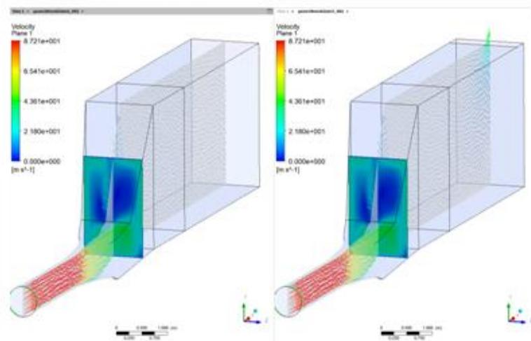
**Figure A6b:- Velocity contours through the HRSG for open end and open topped cases (central plane).**
