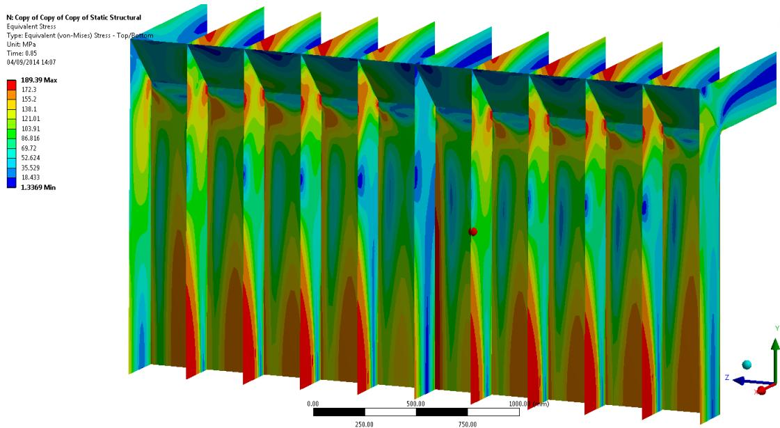
**Figure 6:- HRSG stress analysis (Von Mises Criteria) for static load of 8.5 barg.**
