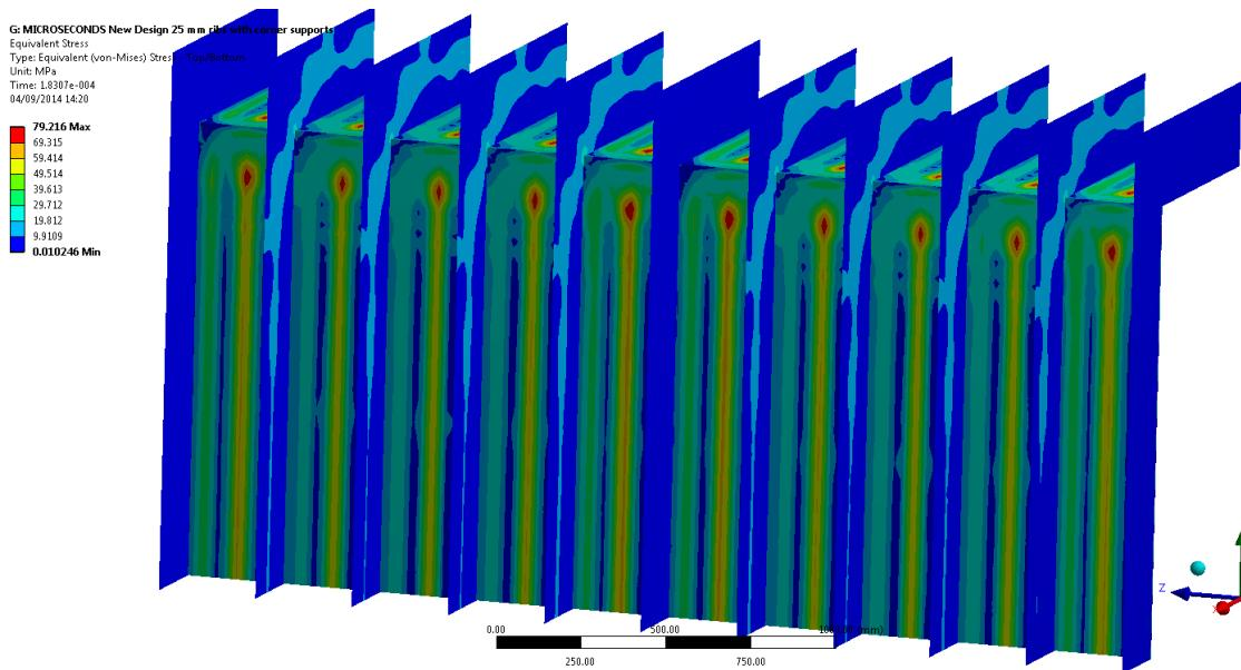
**Figure 8:- HRSG stress analysis (Von Mises Criteria) for a dynamic load of 104 barg.**
