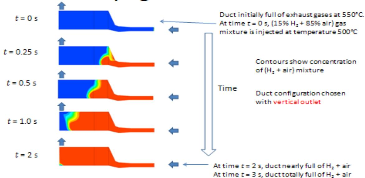
Figure A9a:- Time varying gas concentrations for the open topped case.
