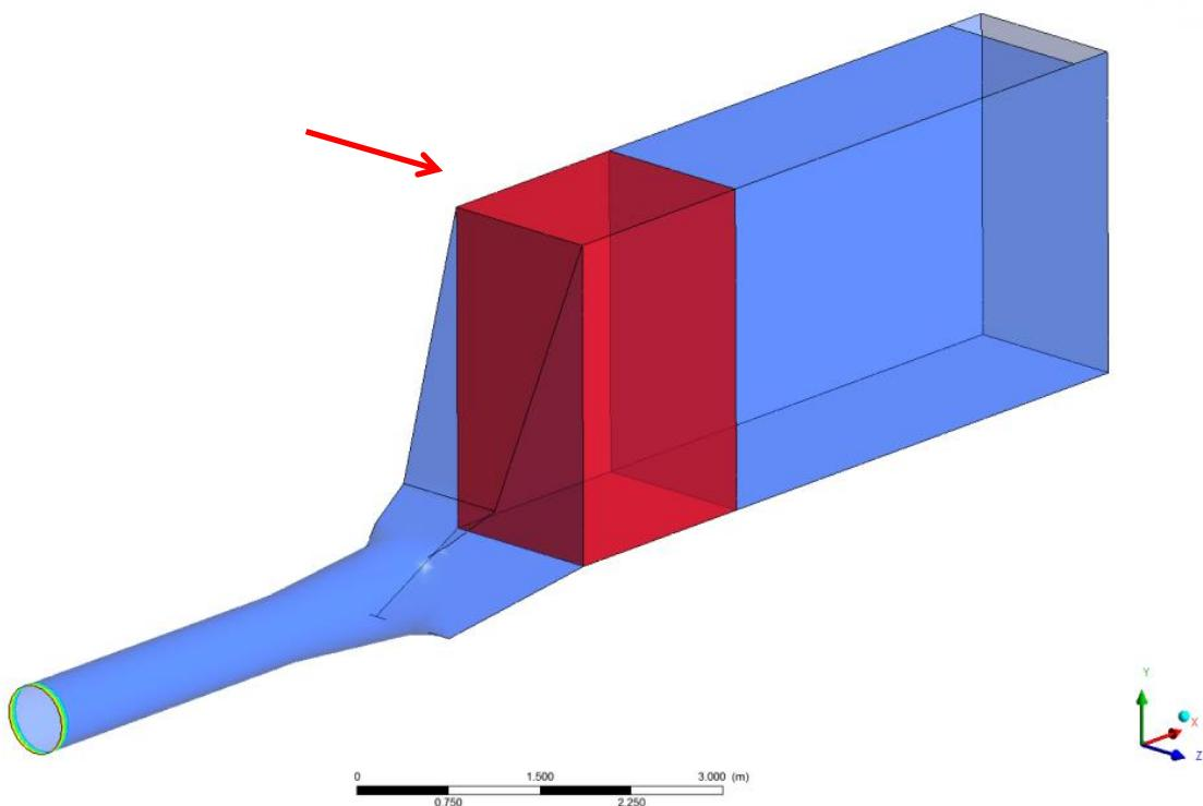
**Figure A3:- Area of model porous region that represents the tube bank (15 rows).**
