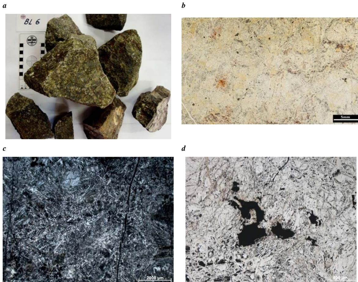
**Figure 34. Photographs of ET6 serpentinite: a) selection of hand specimen fragments; b) scanned polished thin section; c) crossed polarised light photomicrograph showing mesh texture serpentinite hosting several bastite crystals; d) plain light photomicrograph showing black, altered holy-leaf chromite within mesh serpentinite.**
