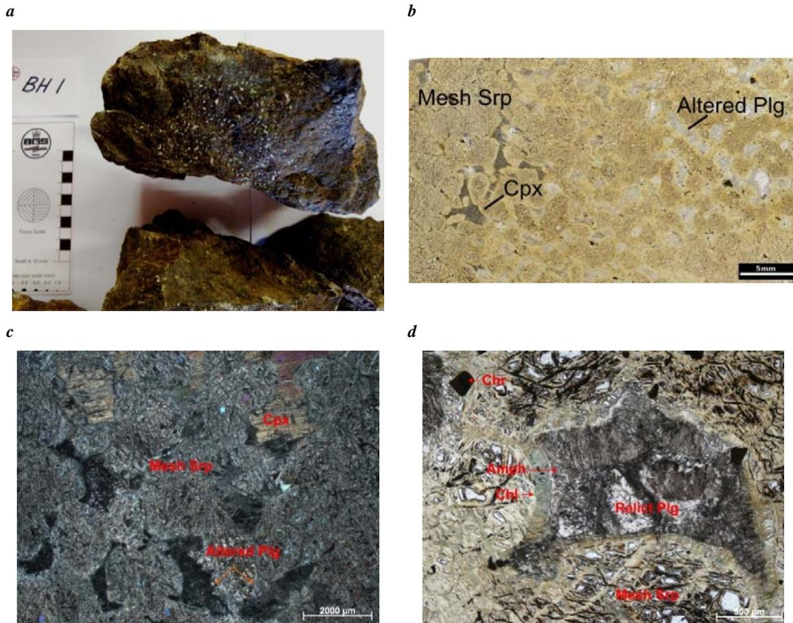
Figure 37. Photographs of ET7 serpentinised plagioclase-rich wherlite showing: a) hand specimen with distinctive white patches of altered plagioclase; b) scanned polished thin section; c) crossed polarised light photomicrograph showing poikilotopic clinopyroxene and interstitial altered plagioclase within a groundmass of serpentinised olivine; d) plane polarised light photomicrograph showing chlorite- amphibole corona that occurs between altered plagioclase and serpentinised olivine.
