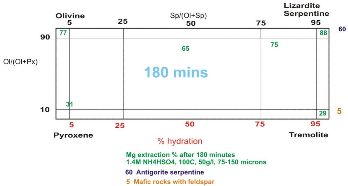
Figure 4. Extraction efficiencies of the tested ultramafic rocks in terms of composition — Reaction time 180 minutes [Copyright BGS, NERC].
