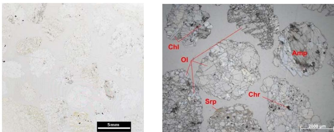
**Figure 66. Scanned polished thin section image and optical microscopy photomicrograph showing the characteristics of the olivine aggregate. The sample contains small amounts of phases, such as: serpentine, chromite, chlorite, amphibole, talc, carbonate, and pyroxene .**
