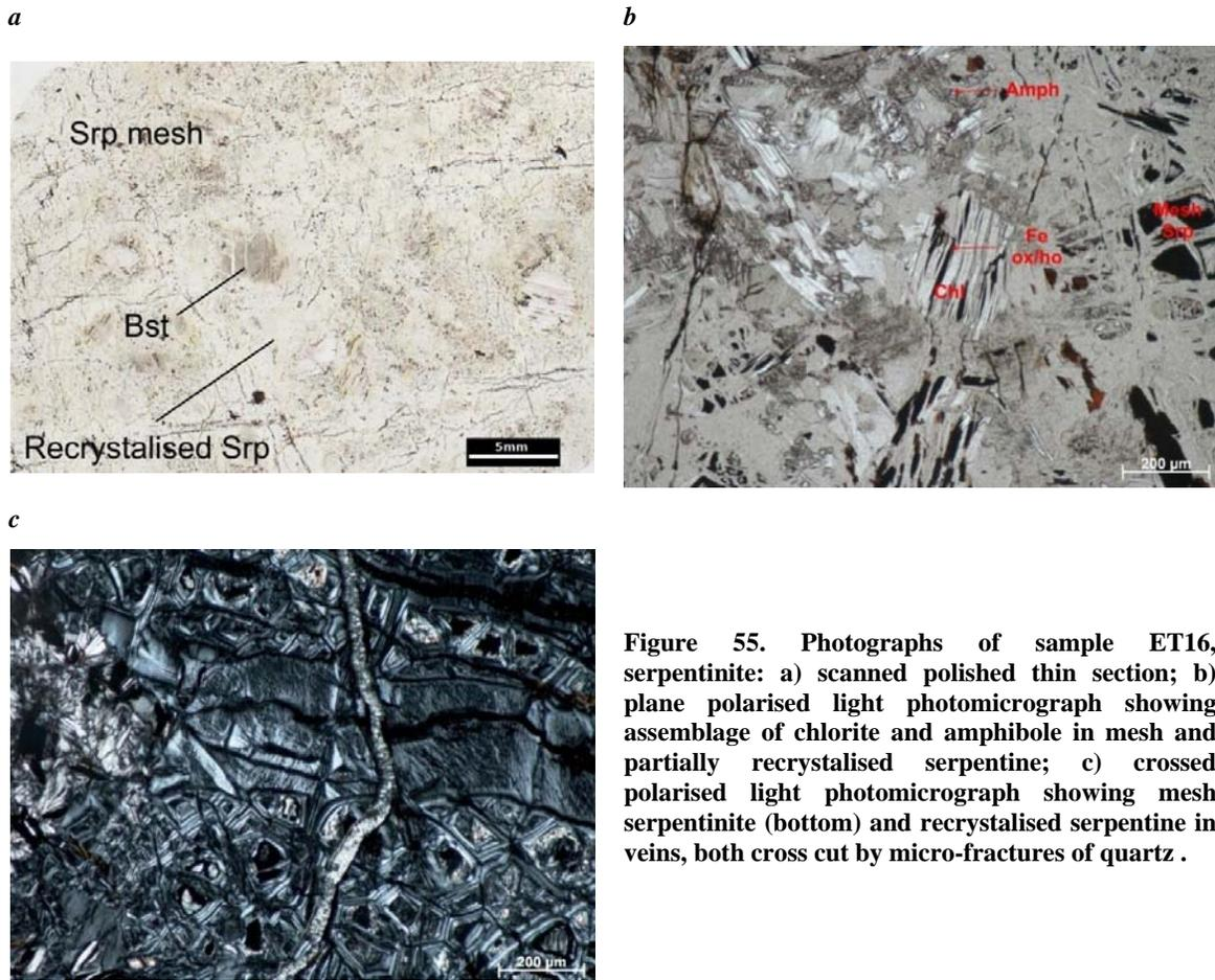
Figure 55. Photographs of sample ET16, serpentine: a) scanned polished thin section; b) plane polarised light photomicrograph showing assemblage of chlorite and amphibole in mesh and partially recrystallised serpentine; c) crossed polarised light photomicrograph showing mesh serpentine (bottom) and recrystallised serpentine in veins, both cross cut by micro-fractures of quartz .
