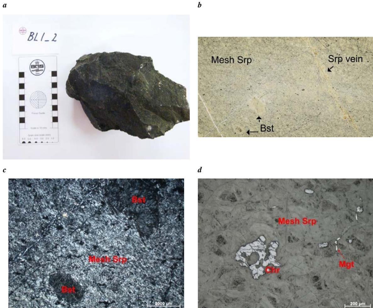
Figure 28. Images of sample ET1: a) hand specimen; b) polished thin section scan; c) crossed polarised light optical photomicrograph showing mesh texture serpentine with scattered large (up to 5 mm) orthopyroxene pseudomorphs – bastites; d) reflected light optical photomicrograph showing crystal of chromite with embayed crystal edges (holly-leaf texture). Minute (<5 µm) fractures of magnetite were commonly observed crosscutting the chromites
