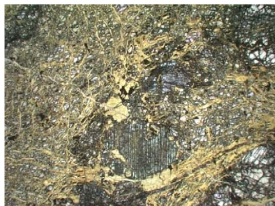
**Figure 67.** Scanned polished thin section image (3 cm longer edge) and optical microscopy photomicrograph showing large crystals of pyroxene in a finer matrix of olivine and serpentine .
