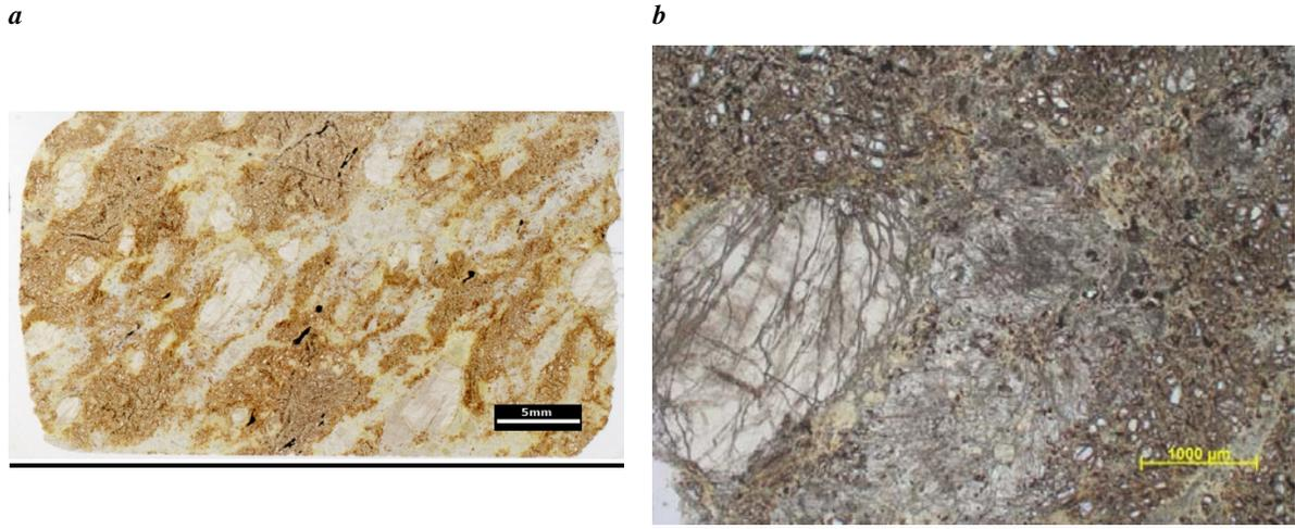
**Figure 59. Photographs of sample ET18, serpentinite: a) scanned polished thin section showing veins; b) plane polarised light photomicrograph showing a large crystal of orthopyroxene adjacent to an aggregate of amphibole after clinopyroxene in a matrix of partially serpentinised olivine. Shetland Area**
