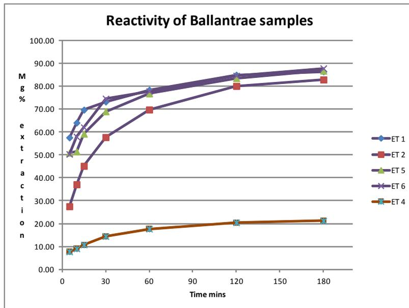
Figure 12. Plot of Mg extraction versus time for the Ballantrae serpentinites (ET 1, ET 2, ET 5, ET 6) and amphibolites (ET 4)
