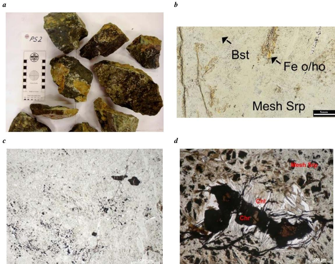
Figure 44. Photographs of sample ET11, chlorite-rich serpentinite: a) hand specimen; b) scanned polished thin section; c) plane polarised light photomicrograph showing mesh serpentine, patchy Fe oxide/oxyhydroxide and scattered chromites; d) plane polarised light photomicrograph showing crystals of chromite rimmed with bladed crystals of chlorite, all within mesh serpentine .
