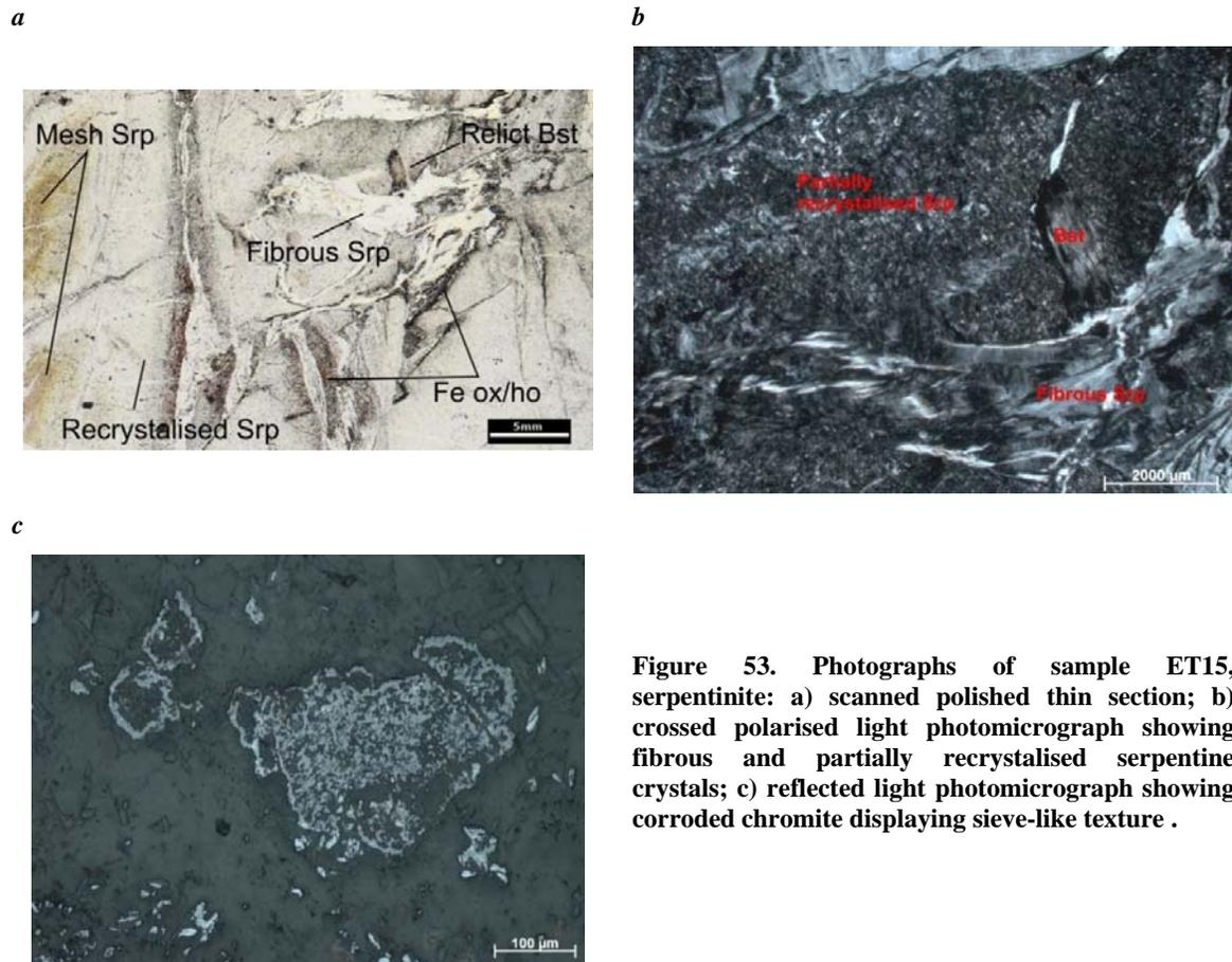
Figure 53. Photographs of sample ET15, serpentinite: a) scanned polished thin section; b) crossed polarised light photomicrograph showing fibrous and partially recrystallised serpentine crystals; c) reflected light photomicrograph showing corroded chromite displaying sieve-like texture .
