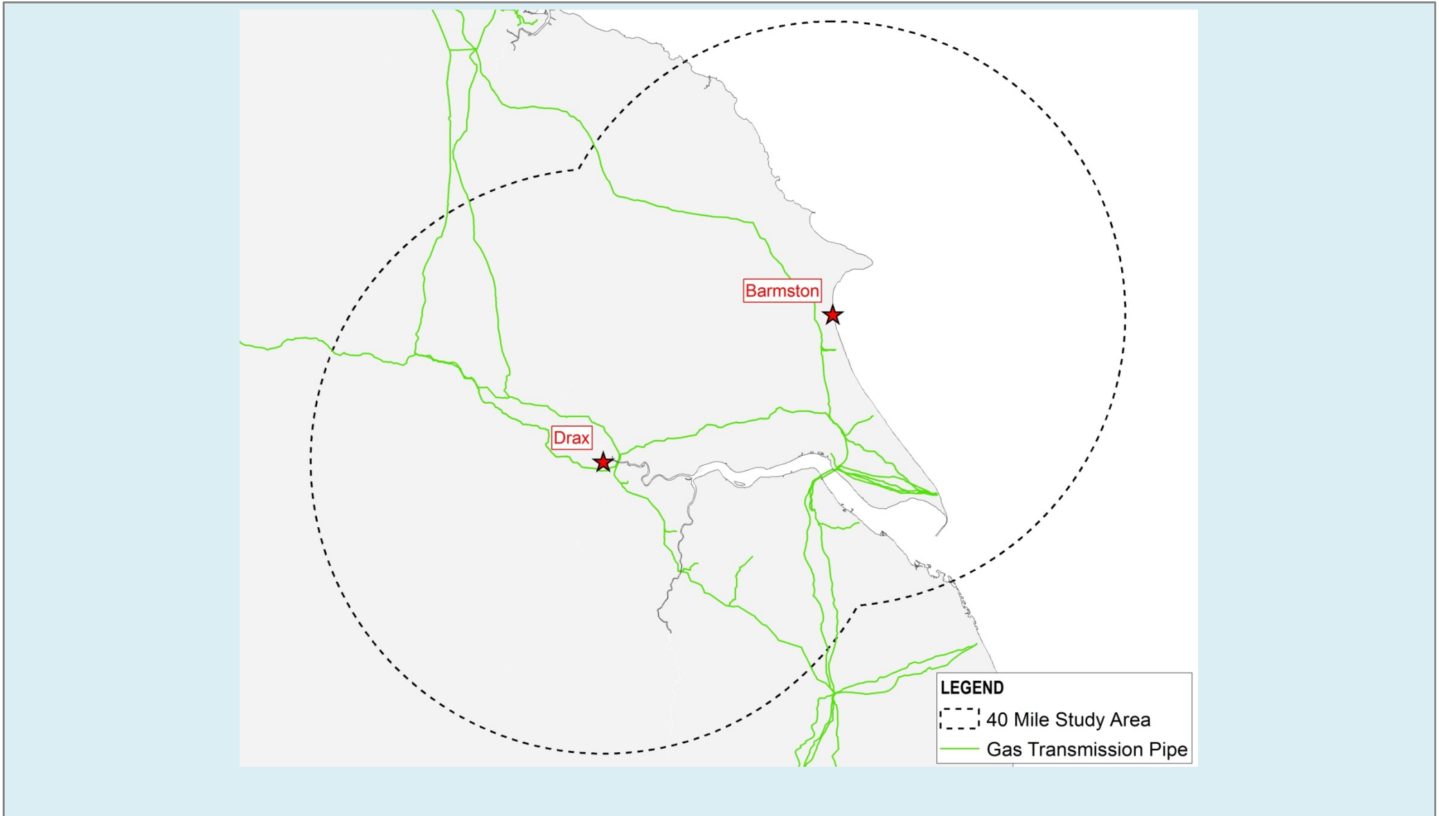
Figure 6 - Gas Supply Network
