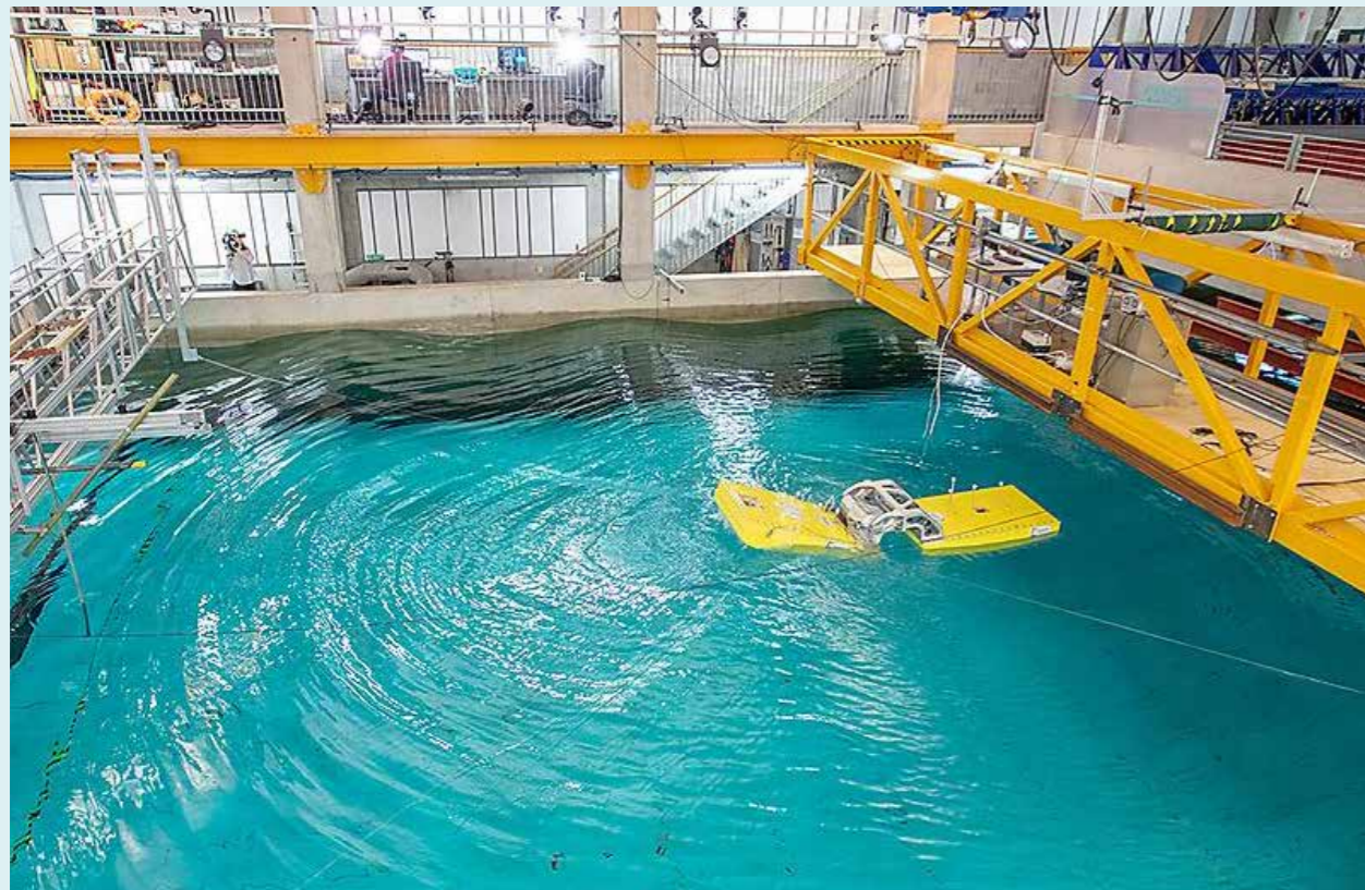
Tank testing at University of Plymouth's COAST Lab (Credit: University of Plymouth)
