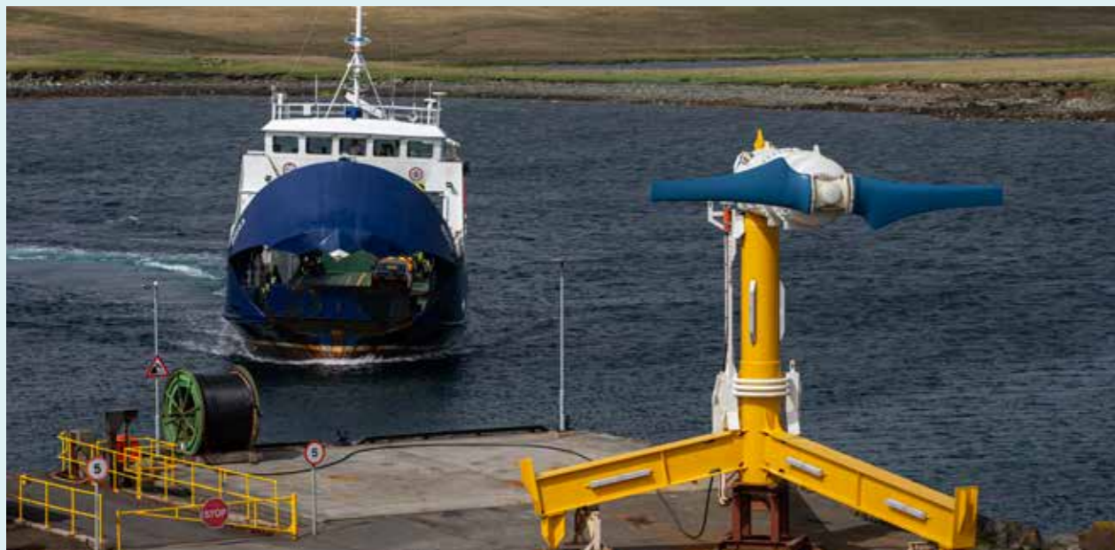
Eunice tidal turbine before deployment (Credit: Nova Innovation)
