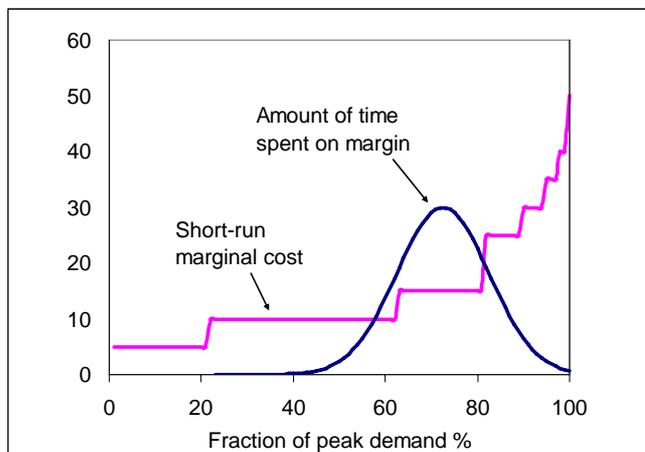
**Figure 2. Schematic merit order for electricity system**
