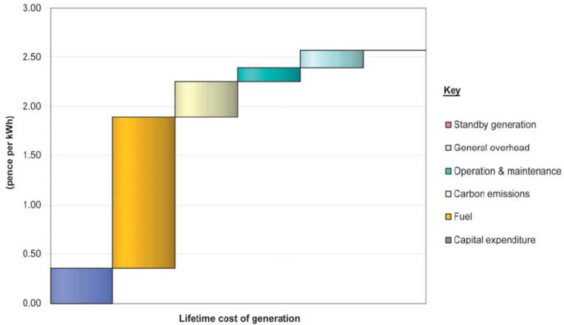
Figure 2.5 LCOE breakdown for CCGT in the mid-2000s
