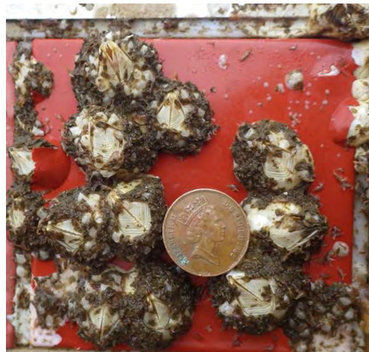
Chirona hameri on FRC coating after 24 months
