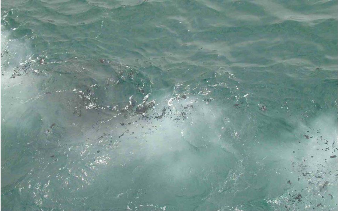
Figure 14. Dispersant in water under oil that is not being dispersed
