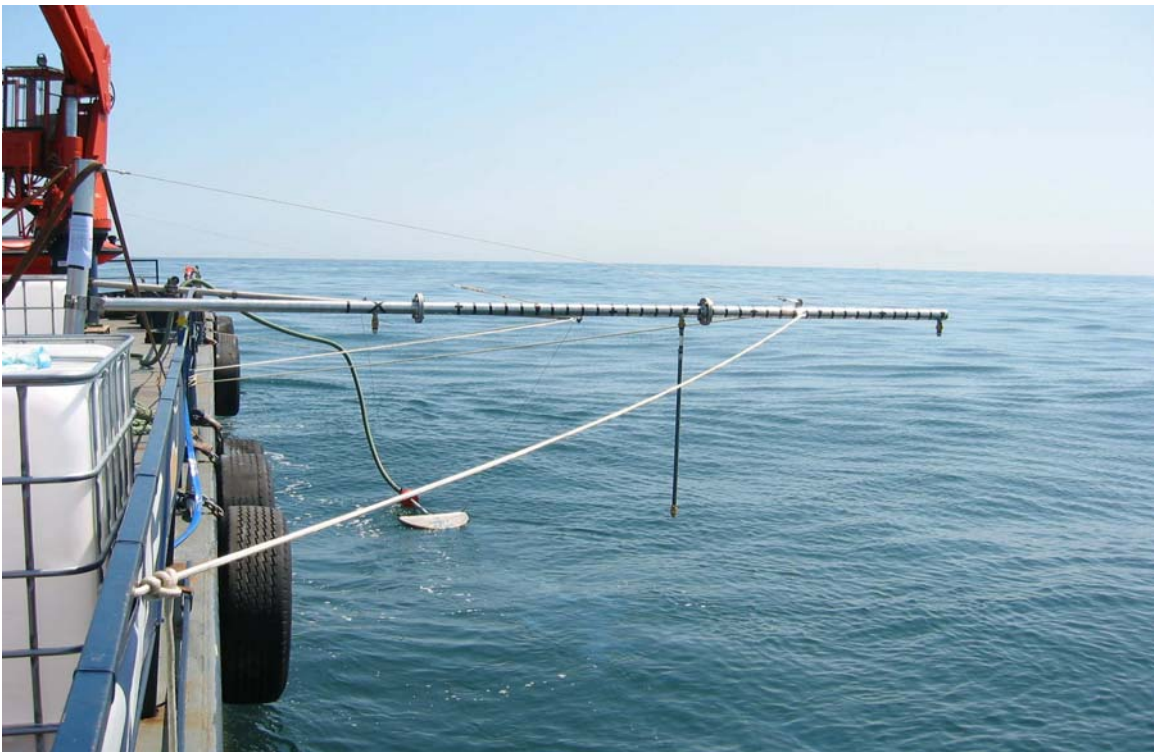
Figure 7 Modified Boatspray system with a single nozzle used to spray dispersants
