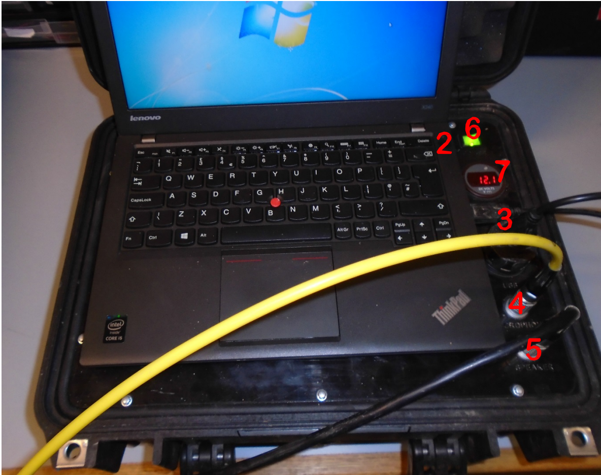
Figure 1 – Taking Measurements – steps 2 to 7 and correct Peli front panel cable connections
