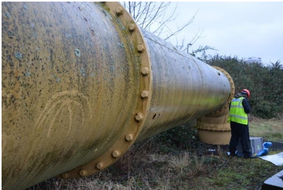
Fig 16. Photograph of the long pipe which is used to measure the sound transmission
