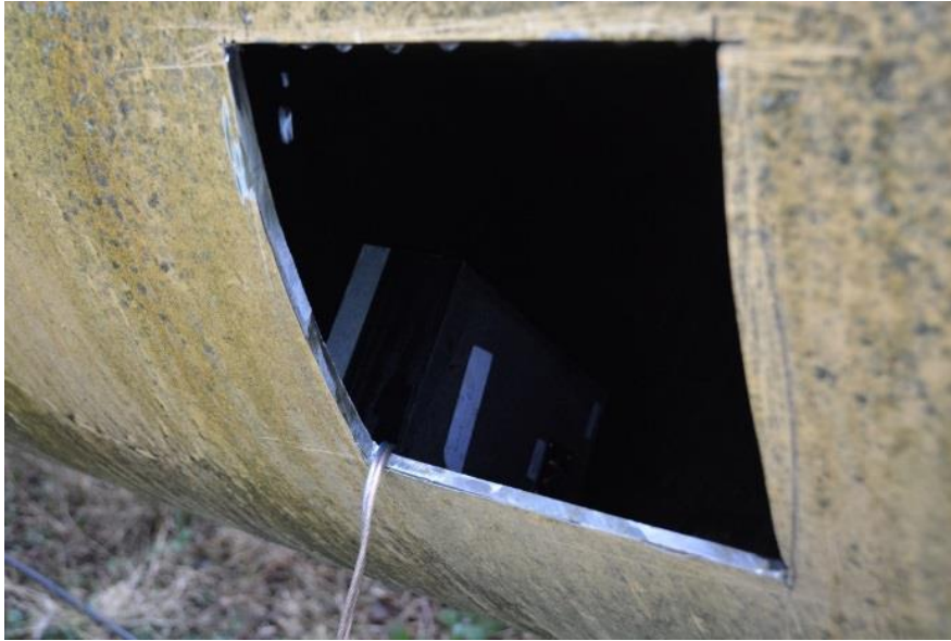
Figure 17. Loudspeaker is used as a source at the one end of the long duct.
