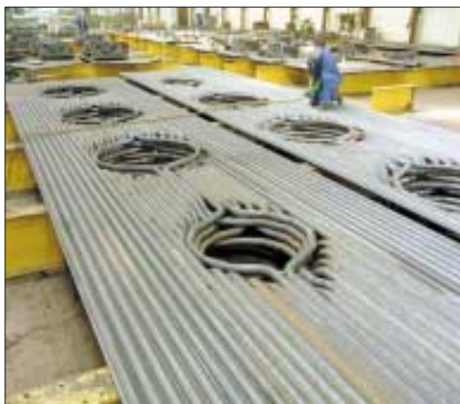
Boiler furnace burner panels
