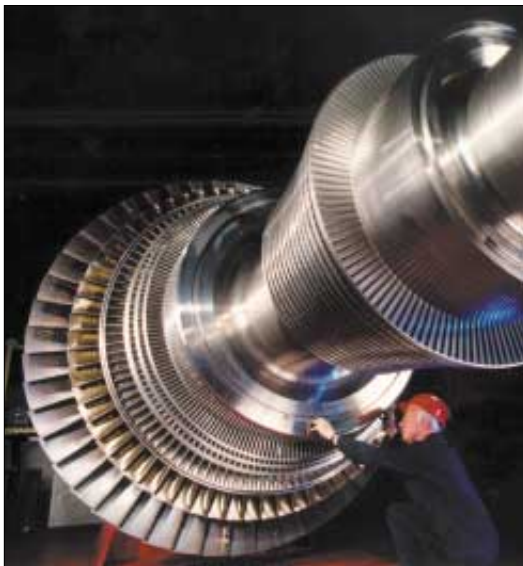
IP/LP turbine rotor (subcritical steam conditions)
