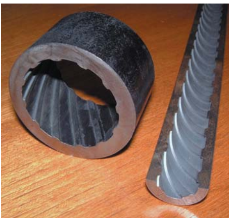
Figure 4. Comparison of regular, (left) and specially optimised ribbed tube
