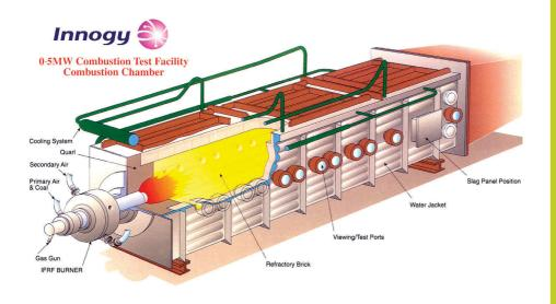
Figure 1. Innogy's 0.5MW Pilot Scale Test Facility
