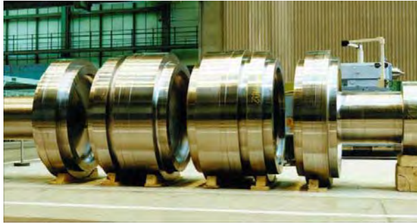
Figure 2.6-14: Forgings for a Typical Welded LP Rotor
