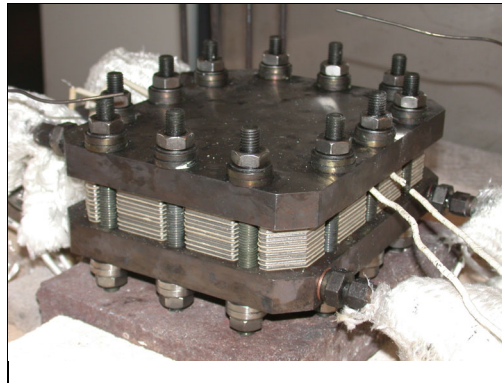
Figure 1: 10-layer Ceres Power short stack prior to testing. This stack delivered 160W e at 600°C.
