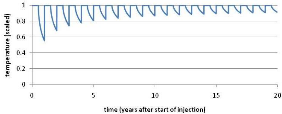
Figure 46 Variation of the well temperature as a function of time. The well temperature decreases during each production phase as fluid from further into the formation migrates towards the production well. The magnitude of this decrease becomes smaller on each cycle as the reservoir overall heats up
