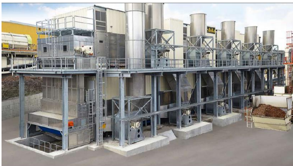
Figure 151: Example of belt dryer arrangement 182
