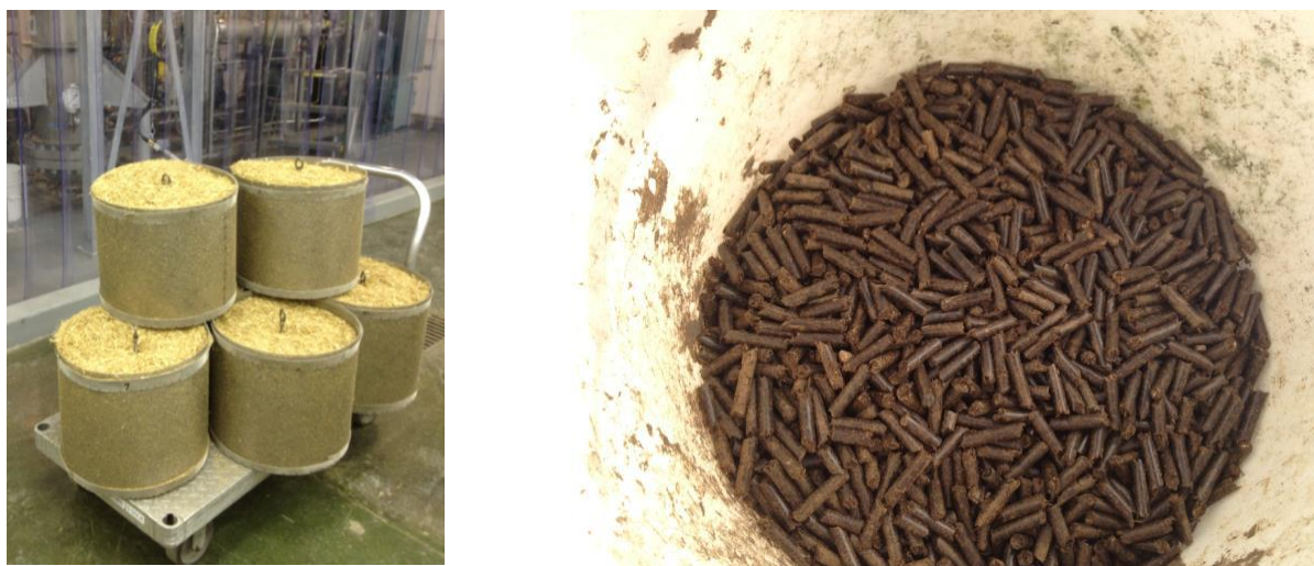
Figure 183: Morphology of untreated corn stover bales (left) and AFEX pellet product (right) 228
