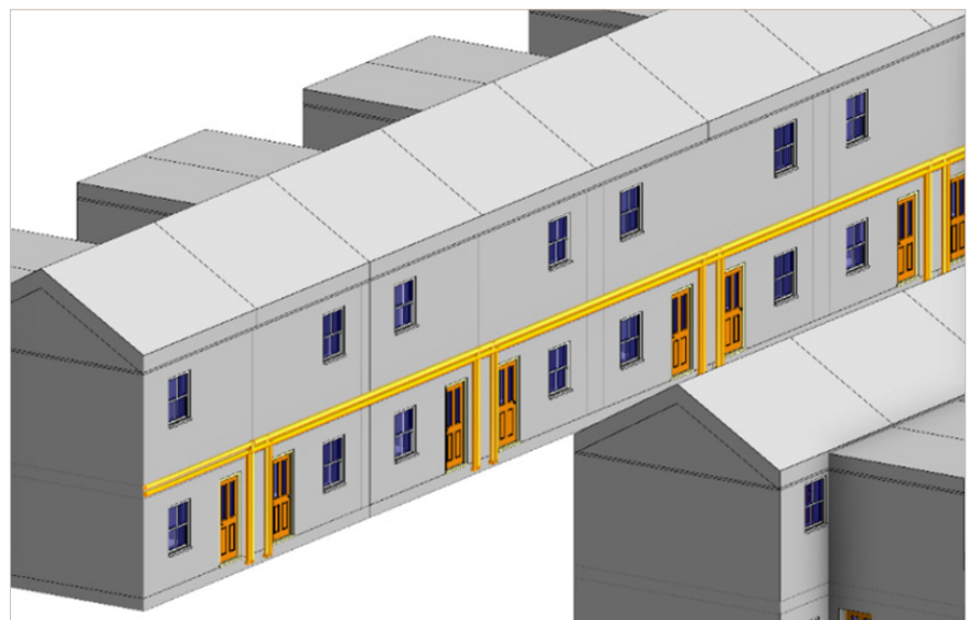
↑ Figure J: Typical arrangement of external wall pipe on front elevation about doorways with entry at ground floor level
