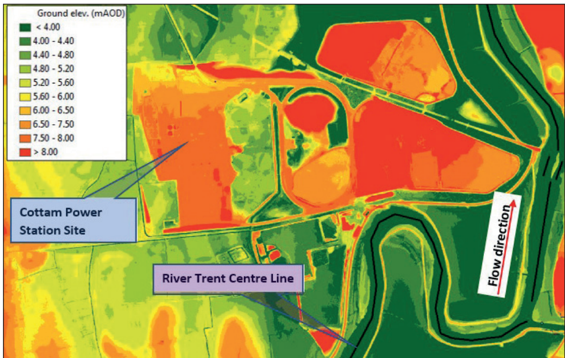
Figure 5. Ground elevation from LIDAR (2011) at Cottam power station site and on the left bank floodplain of the River Trent. (Source: EA)
