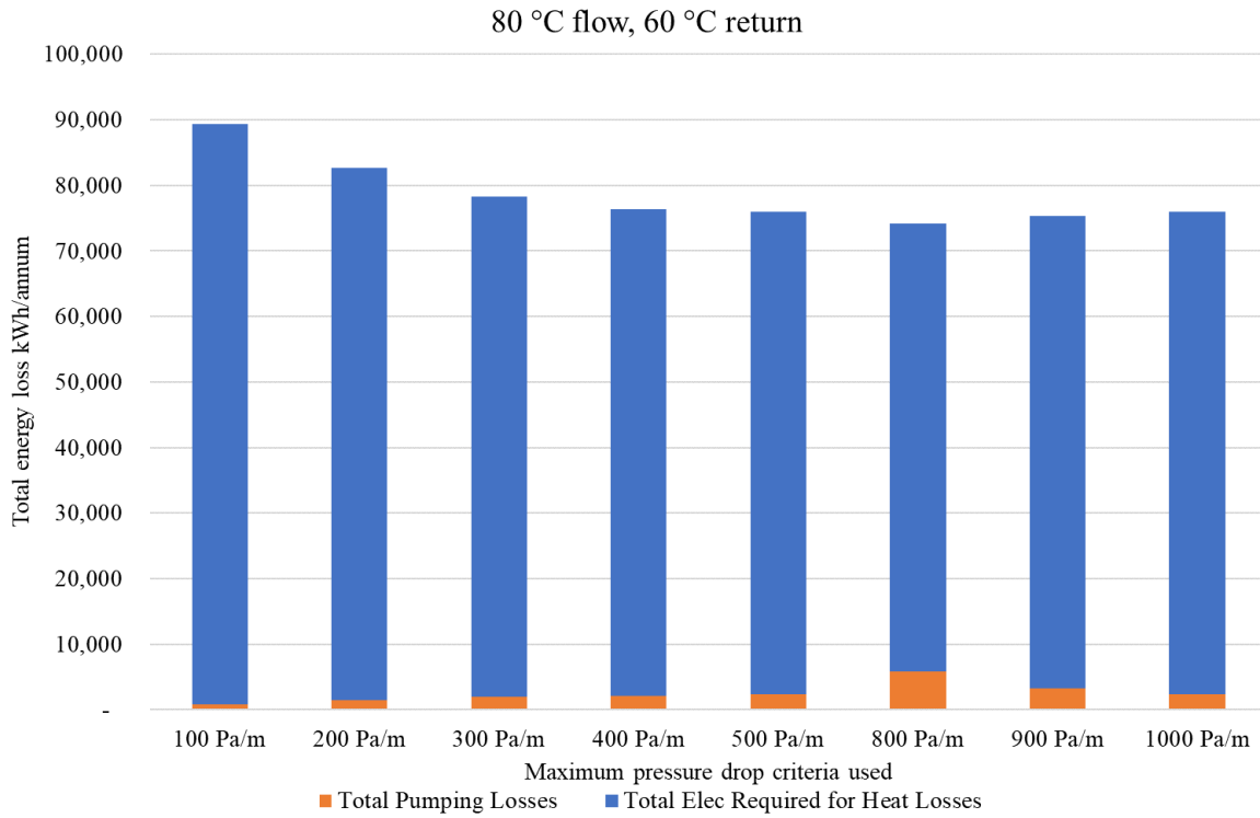
Figure 10 80/60 commercial pipe sizing results
