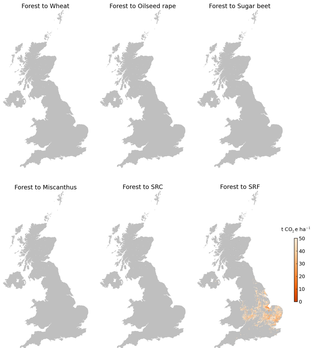
Figure 3.11: Maps showing grid cells with a small positive (detrimental) net GWP (between 0 and 50 t CO 2 e ha -1 ) for the period 2015 to 2050, following conversion from rotational crops, permanent grass and forest to bioenergy crops under the medium climate scenario. The legend shows the colour code of net GWP. Grey represents excluded areas and areas that do not have a small positive net GWP.
