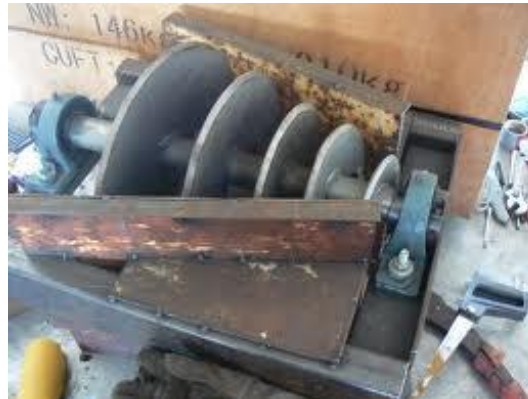
Figure 5-3 Screw chipper (Chipper-Knife)
