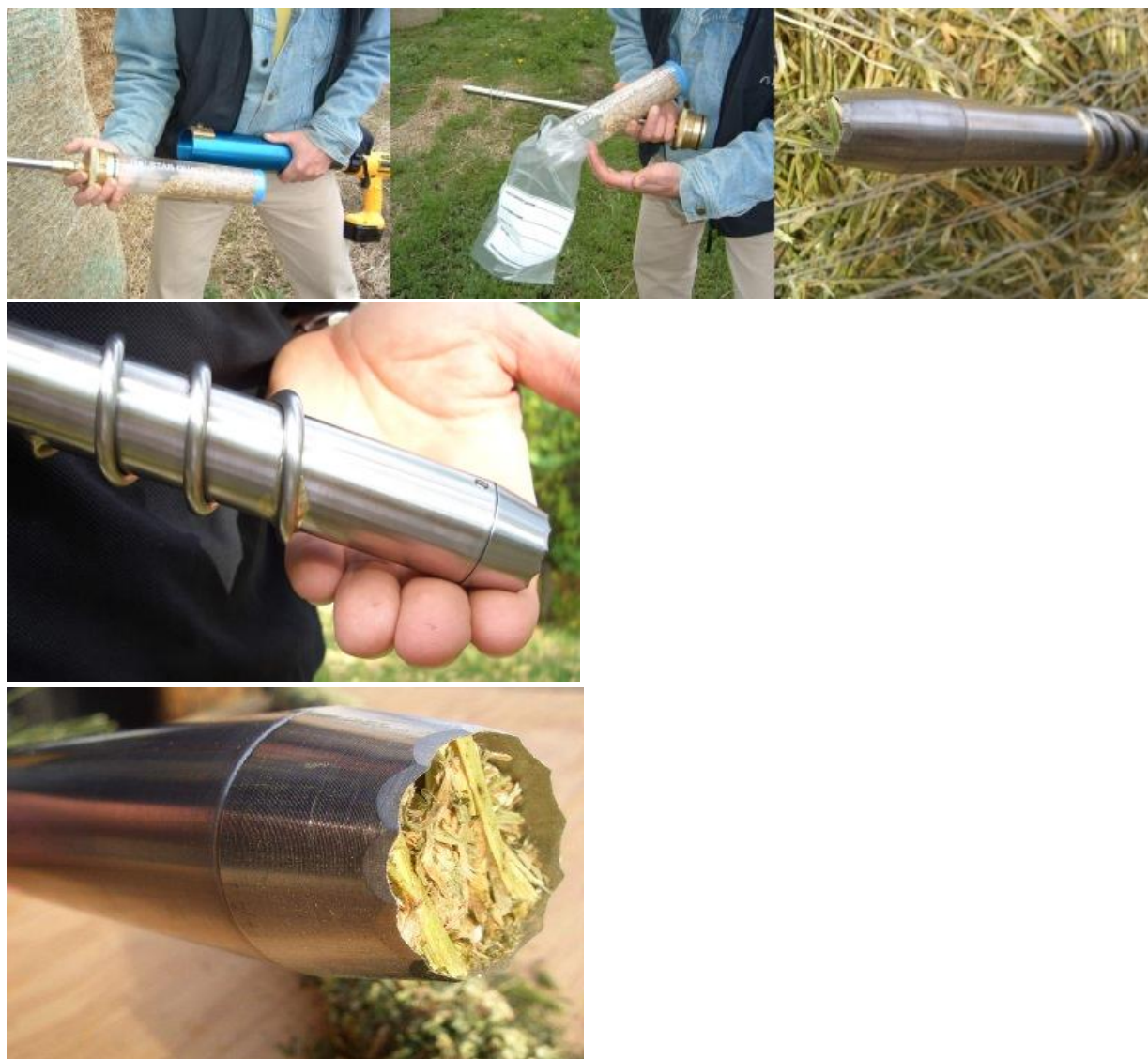
Figure 1: Corer, showing aluminium collection canister with inner, spiral assist and star cutting tip
