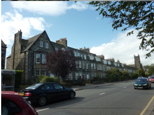
Pre-1919 terraced properties of solid stone construction near Inverleith Gardens. Note rooms-in-roof, dormers and bay windows tend to characterise the architectural style.
