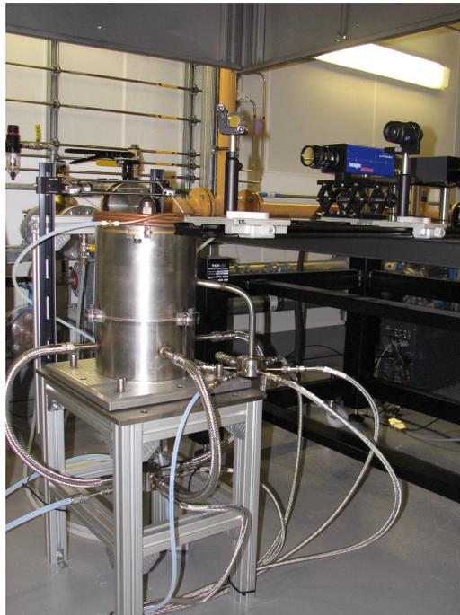
Fig. 2: Photograph of the lifted flame burner
