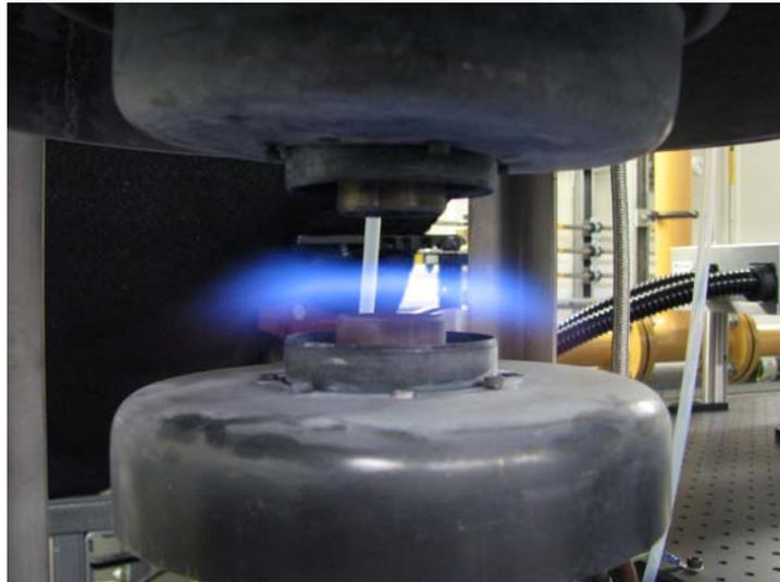
Fig. 34: Typical flame position of the reactants injected from the upper nozzle stabilised against the hot combustion products emerging from the lower nozzle.
