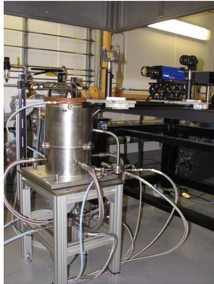
Fig. 7: Photograph of the lifted flame burner
