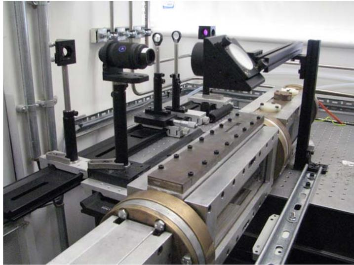
Fig. 53: Optical section of the flame tube along with the optical setup (final three mirrors, telescope and light sheet optics).
