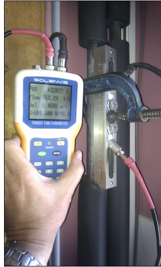
Figure 19: Photograph of the Solenis SL2 in operation, with the transducers in the background.
