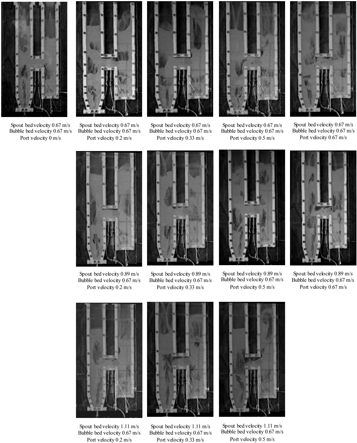
Figure 8 Effect of changing fluidising velocities of the fluidisation of the 2-D model
