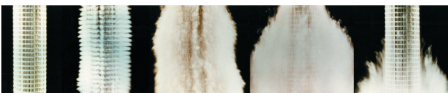
Figure 2. High speed photography showing the action of pulsed jet cleaning
