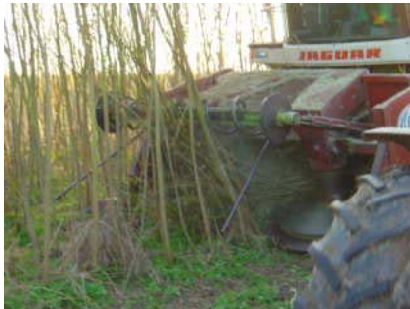
Fig 17 Setting into opened out SRC rows
