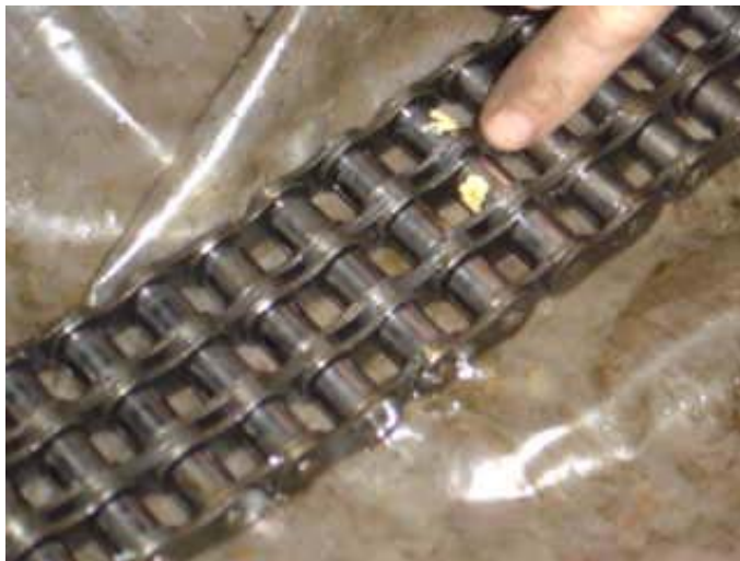
Fig 3 Triple band drive chain added
