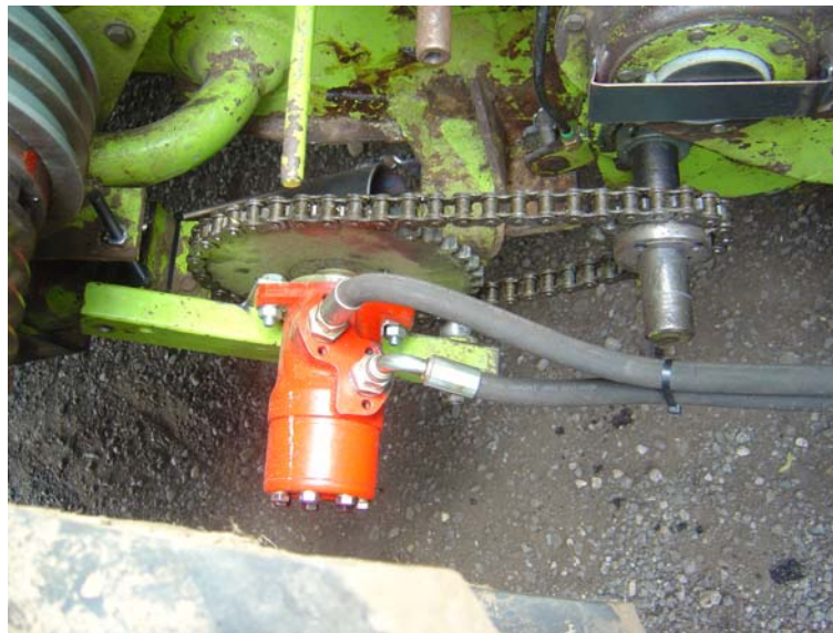
Fig 32 Top view of hydraulic drive
