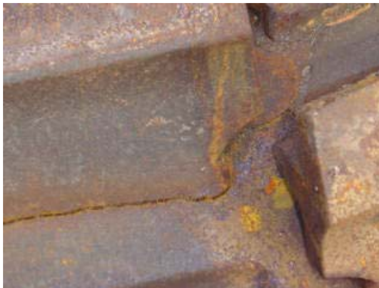
Fig 30 Cracked main chipping drum
