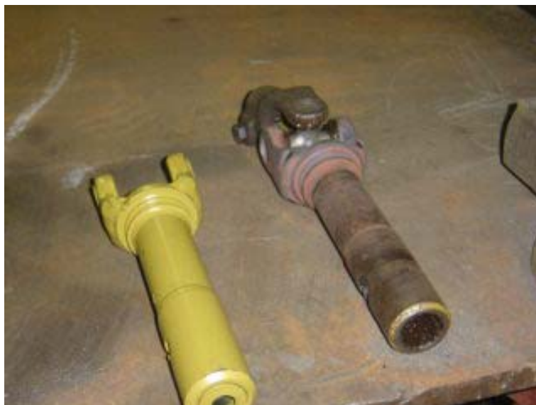
Fig 28 New vs. "worn" drive shaft.
