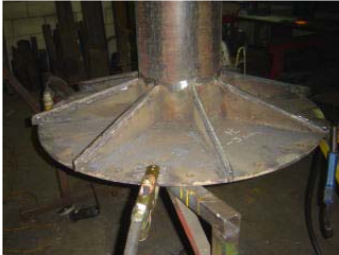
Fig 12 Blade holder assembly
