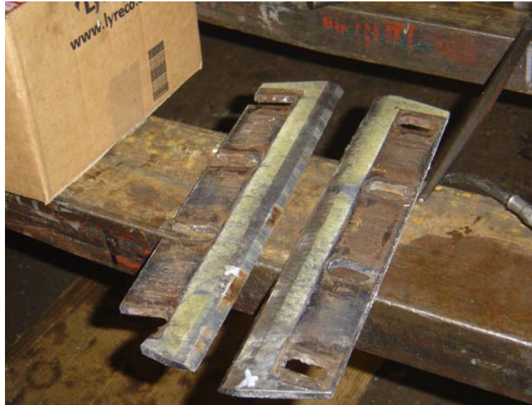
Fig 29 Broken blade corner (left blade)
