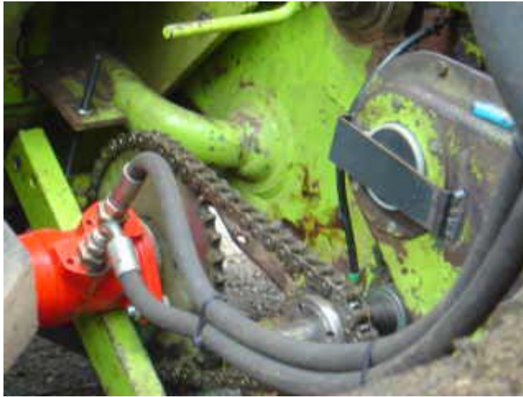
Fig 31 front \frac{3}{4} view of hydraulic drive
