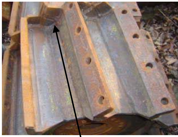
Fig 36 Central spine strengthening plates
