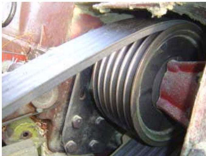
Fig 4 Six groove pulley and powerband
