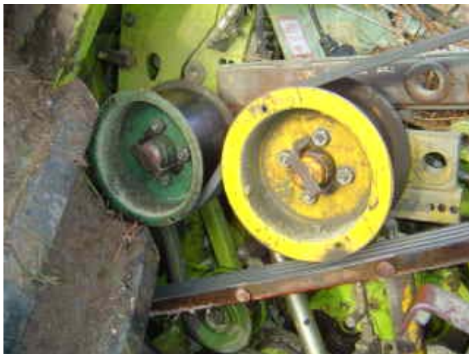
Fig 8 The smoothed out "S" Drive configuration
