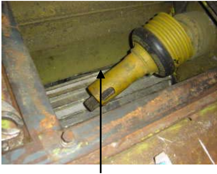
Fig 27 Damage to feed rollers (depression in grooves)
