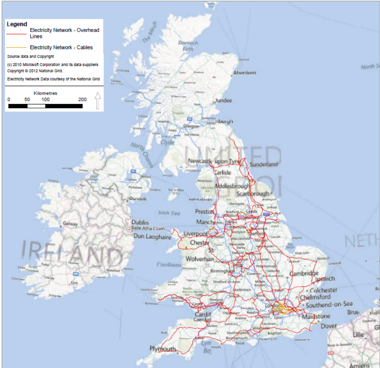
Figure 4—3: National Grid electricity transmission network for England showing overhead lines (red) and cables (yellow).
