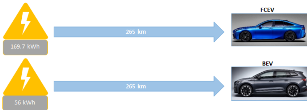
Figure 4-3 Comparison of energy requirements for a hydrogen fuel cell vehicle (the Toyota Mirai) and a battery electric vehicle (the Skoda Enyaq) (Image adapted from Jaroslav Kmet 17 )
