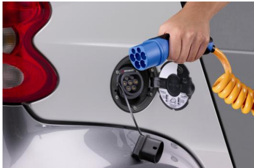
Figure 7: High Visibility Recharging Cable
