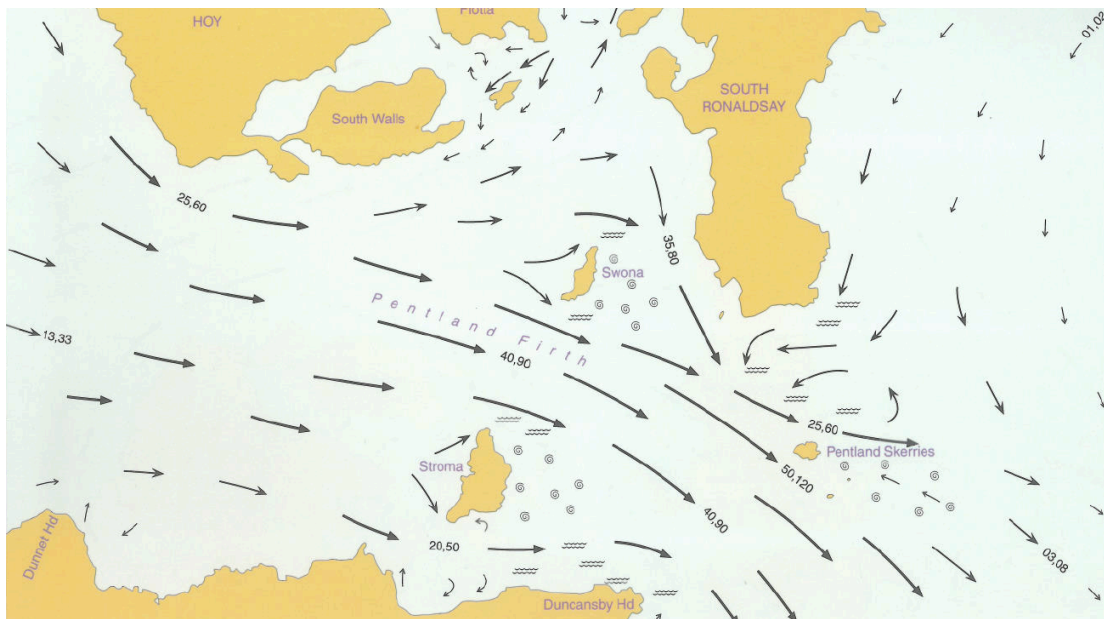
Figure 26 Example of figure from Admiralty Tidal Stream Atlas. Numbers are the current in knots×10 at neap, spring tide
