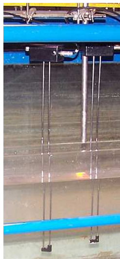
Figure 6 : calibration of the TDH sensors in a basin
