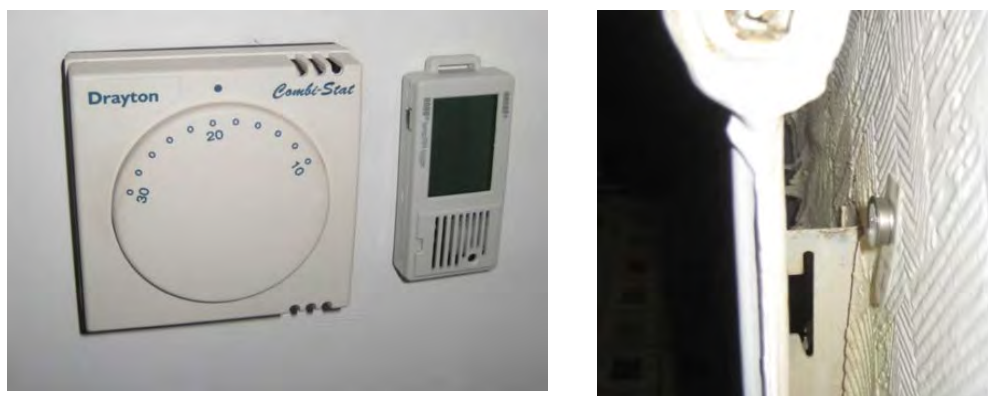
Figure 4: Left, HOBO temperature and humidity sensor mounted to the right of original thermostat. Right, iButton temperature sensor mounted behind radiator. 14
