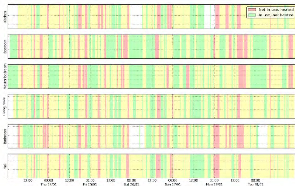
Figure 14: Heating system operation compared to occupancy. Red areas indicate periods when the heating was on but the space was unoccupied, green periods when the heating was not on and the space was occupied. More red areas means more scope for reducing heating system hours of operation, more green areas mean higher potential of increased heating system operation due to take back/rebound.
