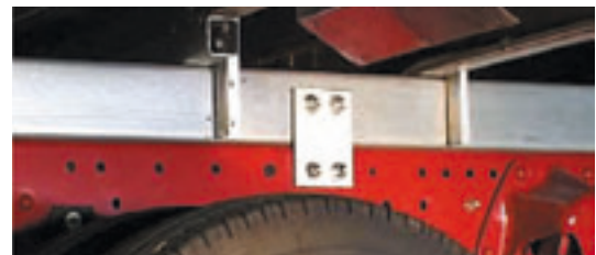
Figure 6 Flexible Front Body Mounting
