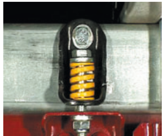
Figure 6 Flexible Front Body Mounting
